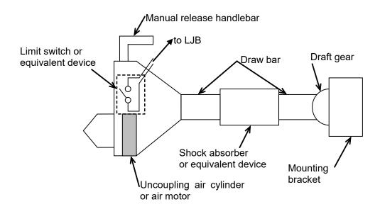
Figure 10.2 Conceptual Illustration of Mechanical Coupler
