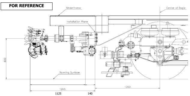
**Figure 10.1 Mounting Dimension of Goods**
