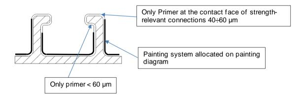
Treatment of rail for fixation of equipment on underframe (Exterior Vehicle)
