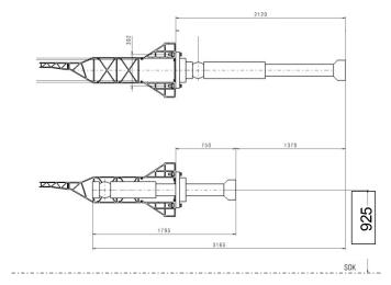
Length from mounting level to coupling level: 2120 mm
