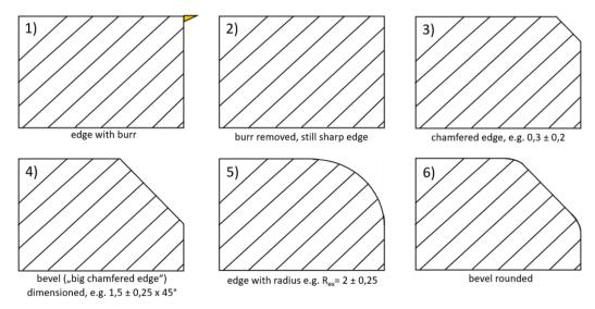
The edge processing in accordance with ISO 13715 must be given on drawings. From the following images, the minimum chamfer values are given
